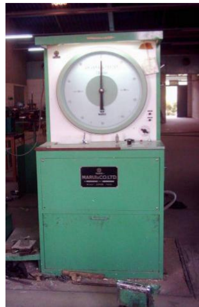
Fig.(3) Loading machine and test setup.
